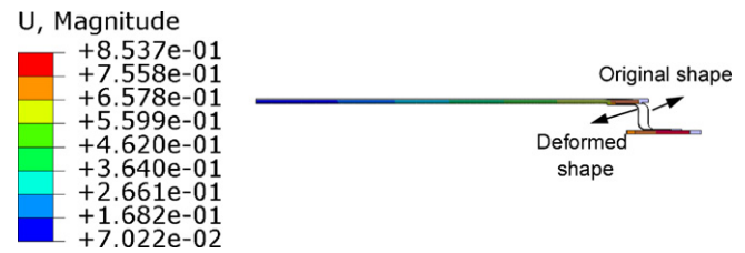
Fig. 14. The bowing deformation.
